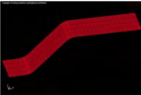
Figure 1. Deformed U-Channel (only half is shown due to symmetric condition)
